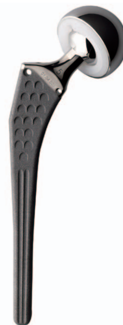
Fig. 1. The Benfix stem is a tapered, rectangular extensive grit-blasted titanium stem with a distal slot.
